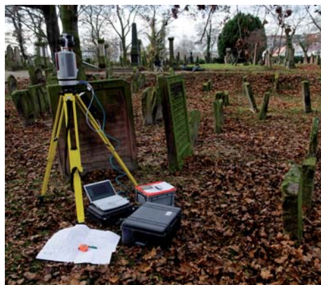
Fig. 3: Installation of the mid-range laserscanning equipment combined with a digital camera for color acquisition. Data acquisition is provided online with RiScanPro running on a Toughbook.
