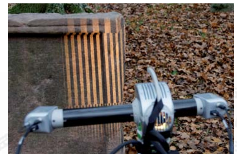
Fig. 4: Close-range 3D-acquisition of the inscription of tombstone Brocke No. 1061 using structured light (also known as coded light).
